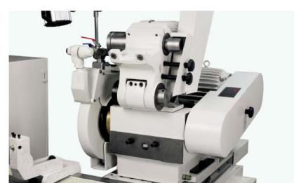
1. Internal Grinding Attachment
