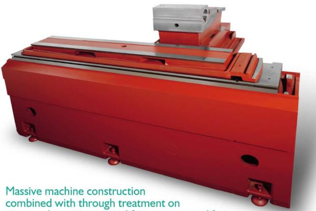
Massive machine construction combined with through treatment on structural parts is a critical factor to assure lifetime accuracy of a grinder. The EXTOMAX series CNC cylindrical grinder is manufactured by an advanced structure design concept and subject to a comprehensive heat treatment. This guarantees consistent accuracy year after year.
